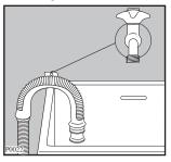
In a sink drain pipe branch. This branch must be above the trap so that the bend is at least 60 cm above the around.
